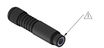
NOTE: 1. MUST BE MANUFACTURED TO STANDARD MALE SMA CONNECTOR DIMENSIONS. B
