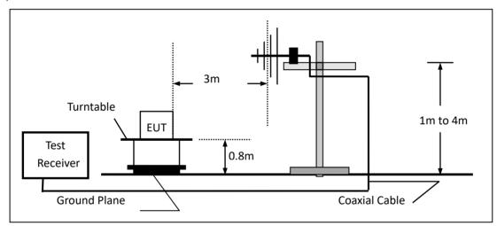
(c) For radiated emissions above 1000MHz
