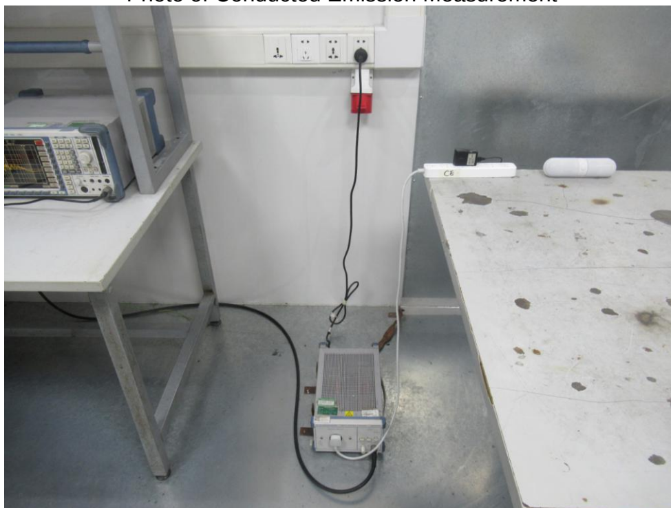
Photo of Conducted Emission Measurement
