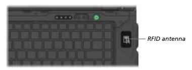
This module is enabled by default. To enable or disable the module, run the BIOS Setup program and select Advanced  $\rightarrow$  Device Configuration  $\rightarrow$  RFID Card Reader. (See Chapter 5 for information on BIOS Setup.)
