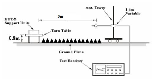
The radiated emission below 1GHz tests were performed in the 10 meters chamber test site, above 1GHz tests were performed in the 3 meters chamber test site B, using the setup accordance with the ANSI C63.4-2014. The specification used was with the FCC Part 15 B Class B limits.
