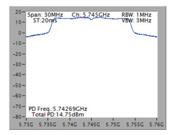
Power Density Plot on Configuration IEEE 802.11ac MCS0/Nss1 VHT40 / Chain 1 + Chain 2 + Chain 3 / 5755 MHz
