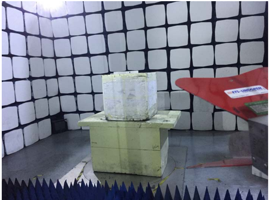
Radiation Emission Test Setup (1GHz to 18GHz)
