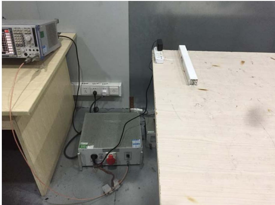
Conducted Emission Test Setup
