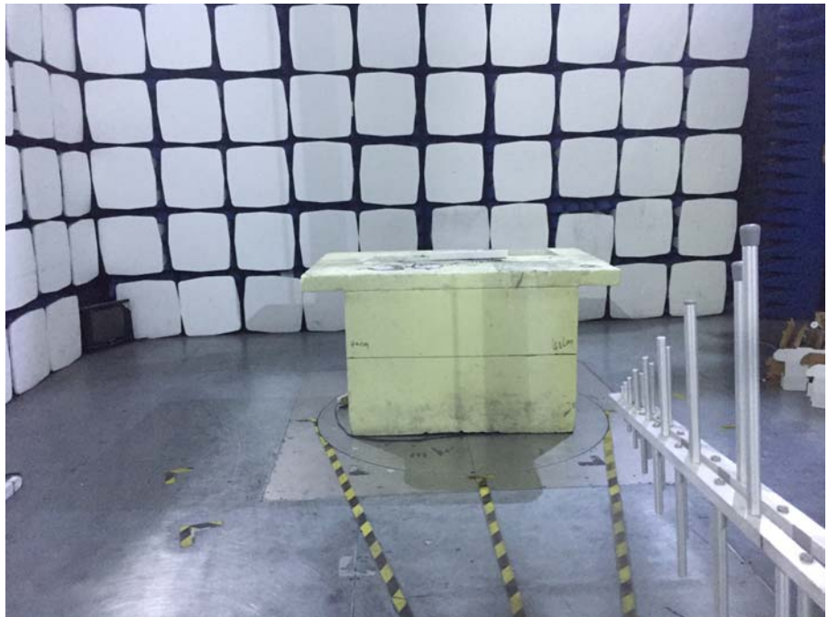
Radiation Emission Test Setup (30MHz to 1GHz)
