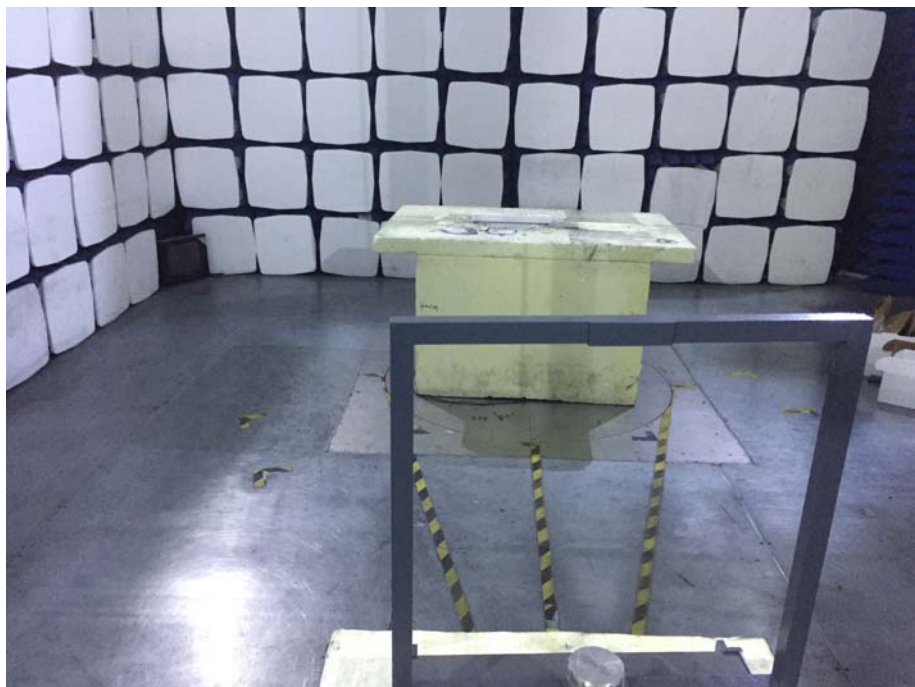
Radiation Emission Test Setup (Below 30MHz)
