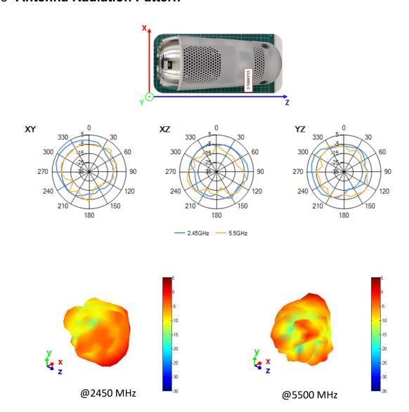
All data is measured while CU23001-1 adhered to the Owl's device.
