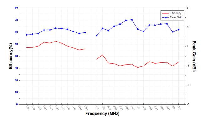
All data is measured while CU23001-1 adhered to the Owl's device.
