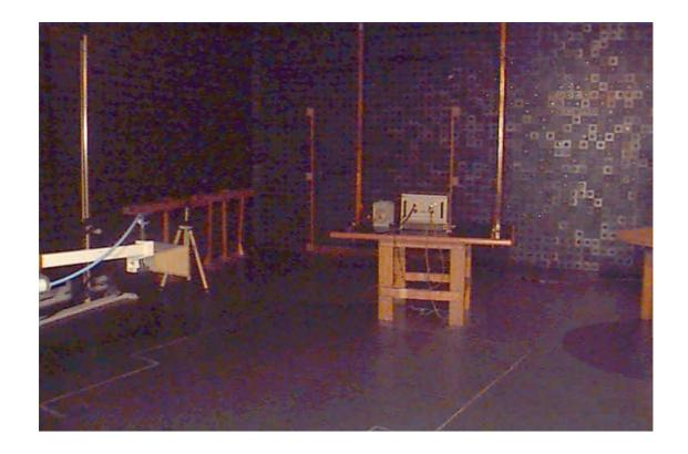
Photograph No.6 Unintentional radiated emissions measurement setup anechoic chamber
