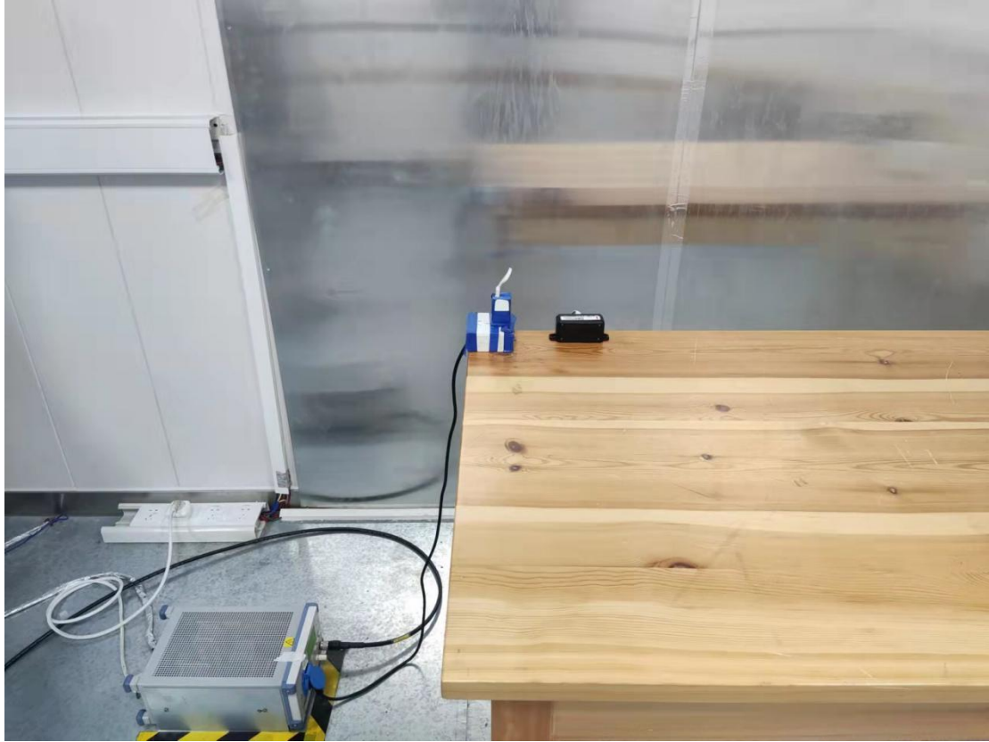
Conducted emission test setup
