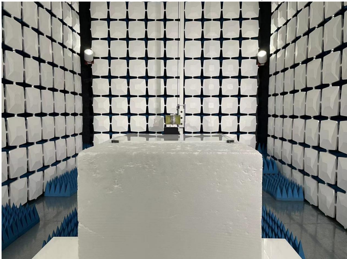
Above 1GHz for radiated emission test setup
