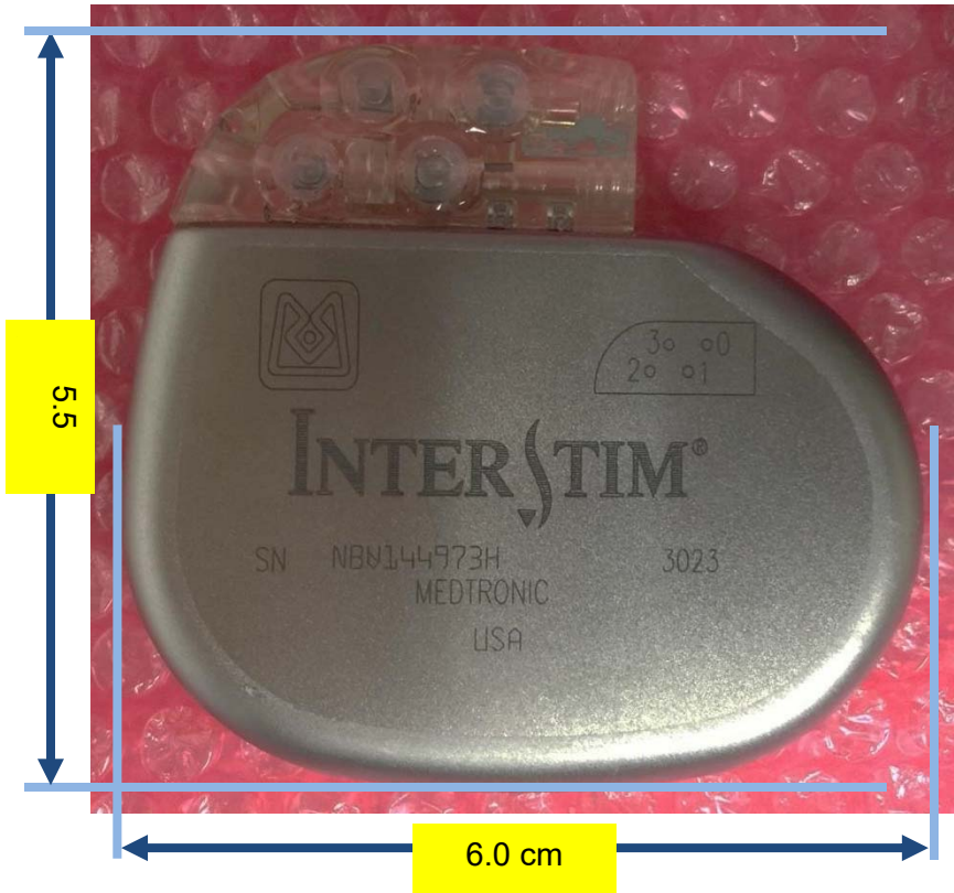
Figure 1: InterStim® , Model: 3023, Front View (with dimensions)
