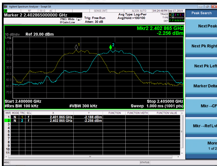
TEST PLOT FOR FREQUENCY SEPARATION
