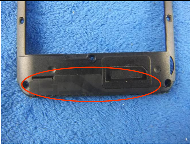
GSM/PCS/UMTS-FDD/LTE Antenna View
