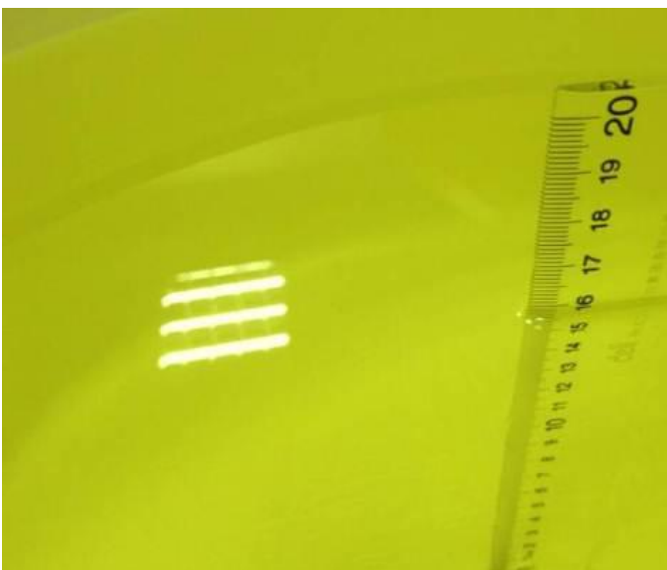
Picture9-2: Liquid depth in the Flat Phantom (1750 MHz Head)
