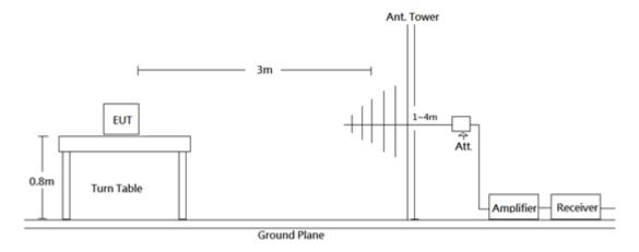
Radiated emission tests were performed in the 3 meters chamber test site, using the setup accordance with the ANSI C63.10-2013. The specification used was the FCC Part 15.209 and FCC 15.225 Limits.
