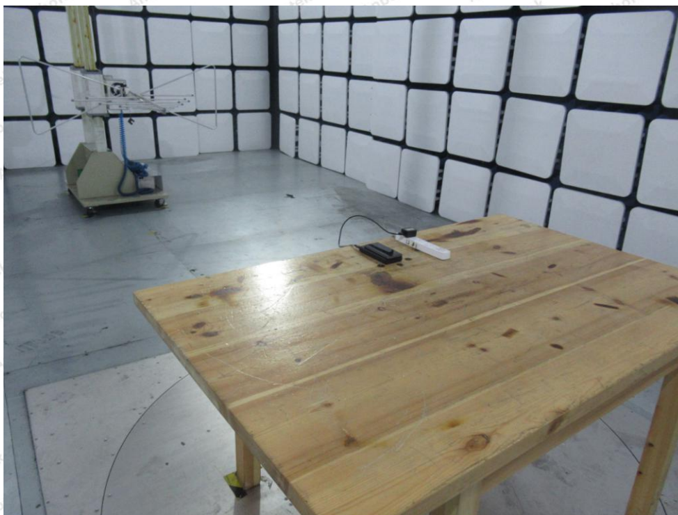
Photo of Radiation Emission Test
