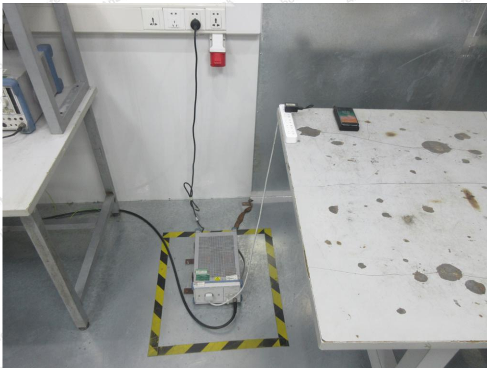
Photo of Conducted Emission Measurement
