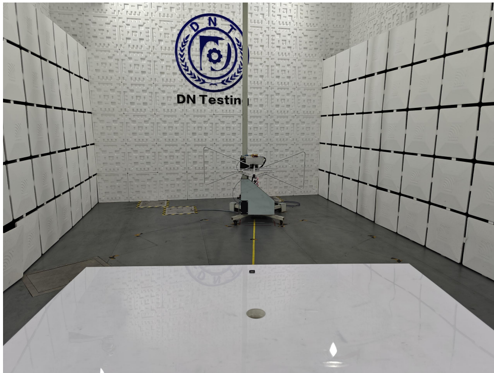
Radiated Emission Test View|(Below 1G)
