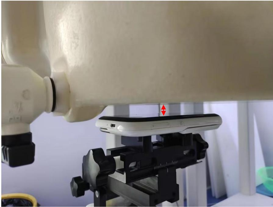
**Face Up Setup Photo (Antenna Open) (10 mm)**
