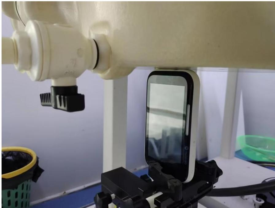
**Handheld Top Setup Photo (Antenna Closed)**
