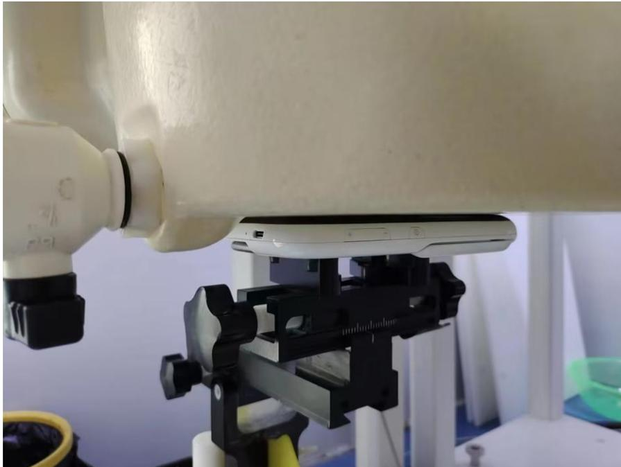
**Handheld Back Setup Photo (Antenna Closed)**
