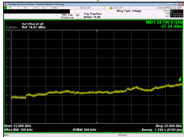
BLE/GFSK 1 Mbps Mid Channel, 2442 MHz
