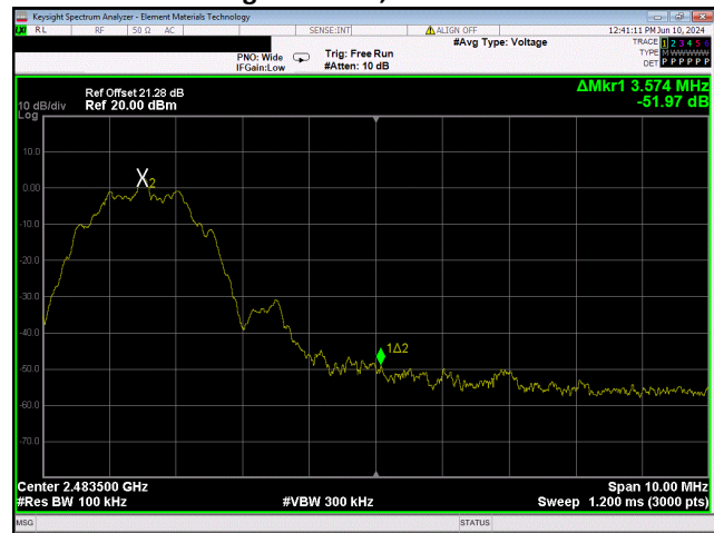
BLE/GFSK 2 Mbps High Channel, 2480 MHz
