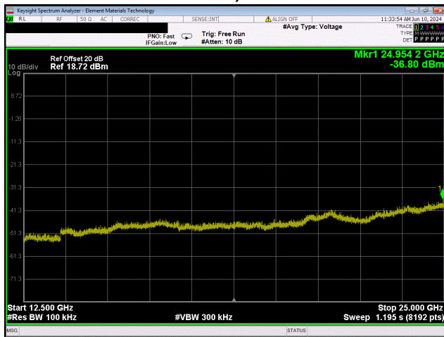
BLE/GFSK 1 Mbps Low Channel, 2402 MHz
