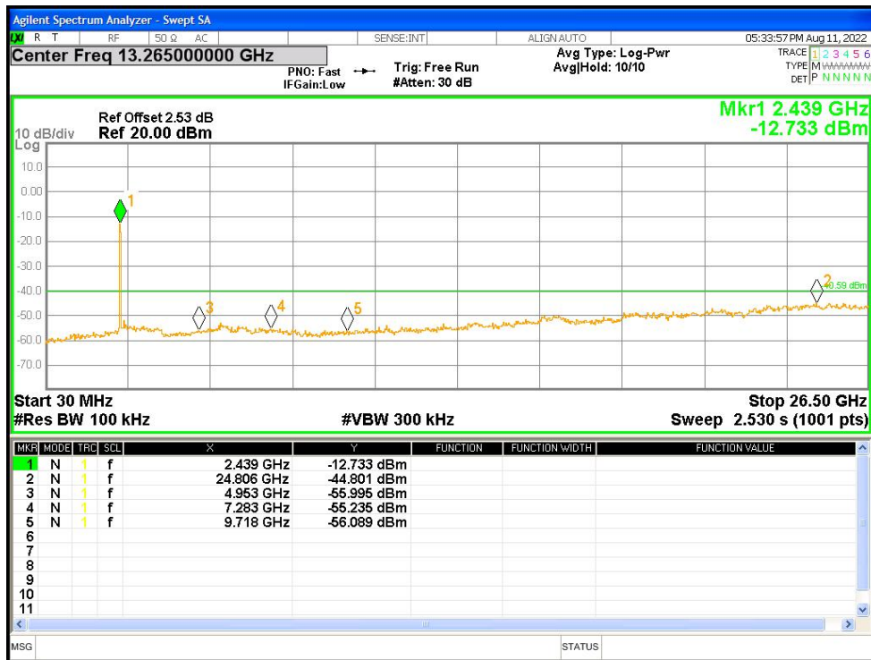
Tx. Spurious NVNT n40 2452MHz Ant1 Ref
