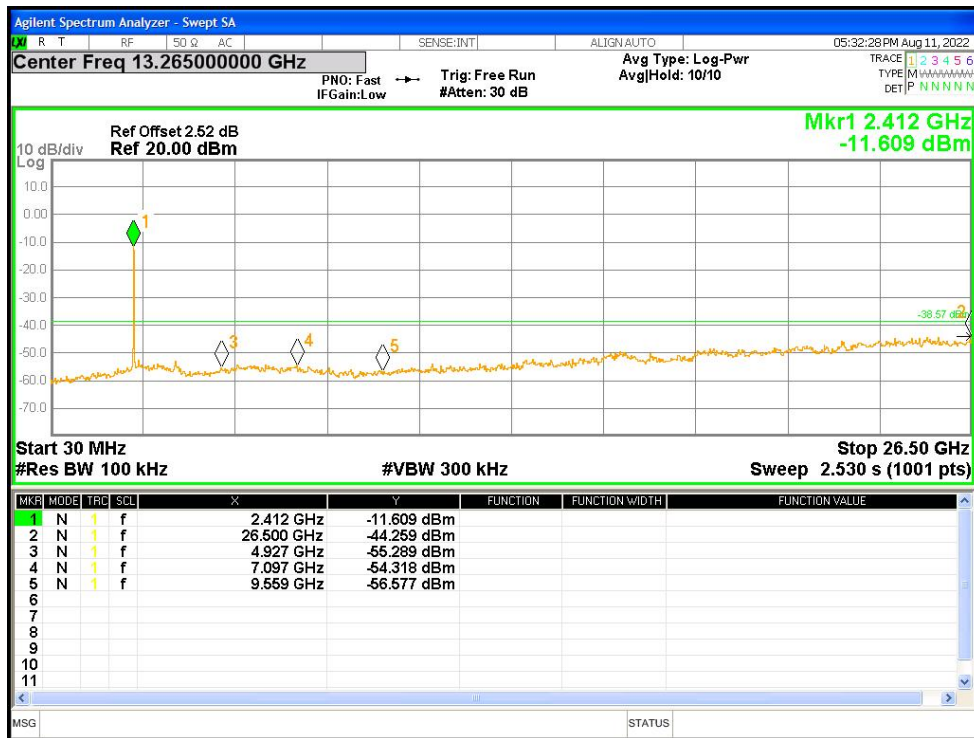
Tx. Spurious NVNT n40 2437MHz Ant1 Ref
