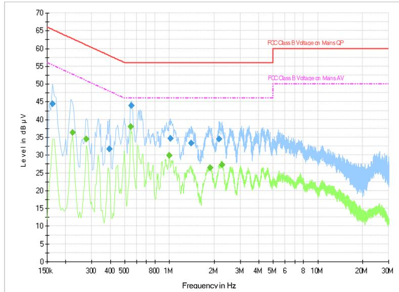
**Fig.B.9.1 AC Powerline Conducted Emission- bluetooth**
