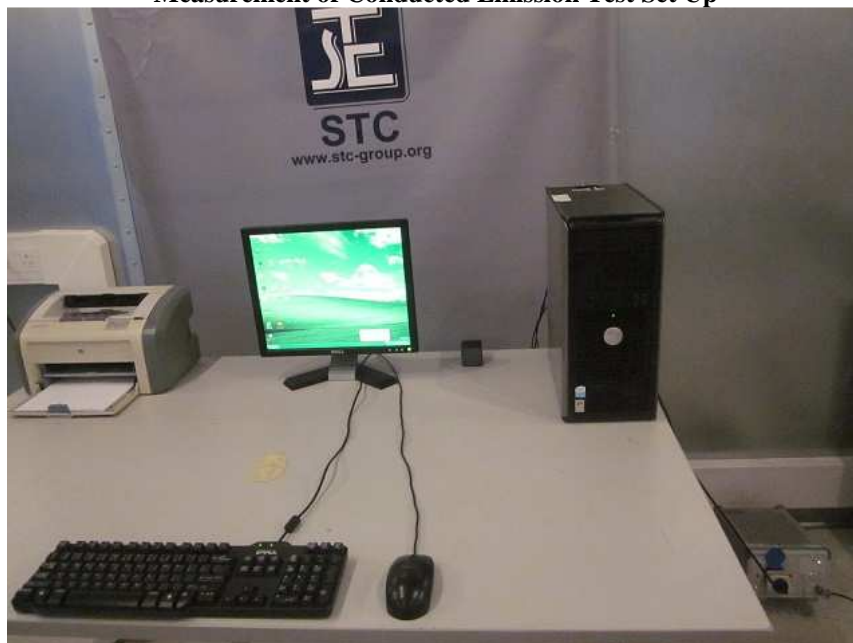
Measurement of Conducted Emission Test Set Up
