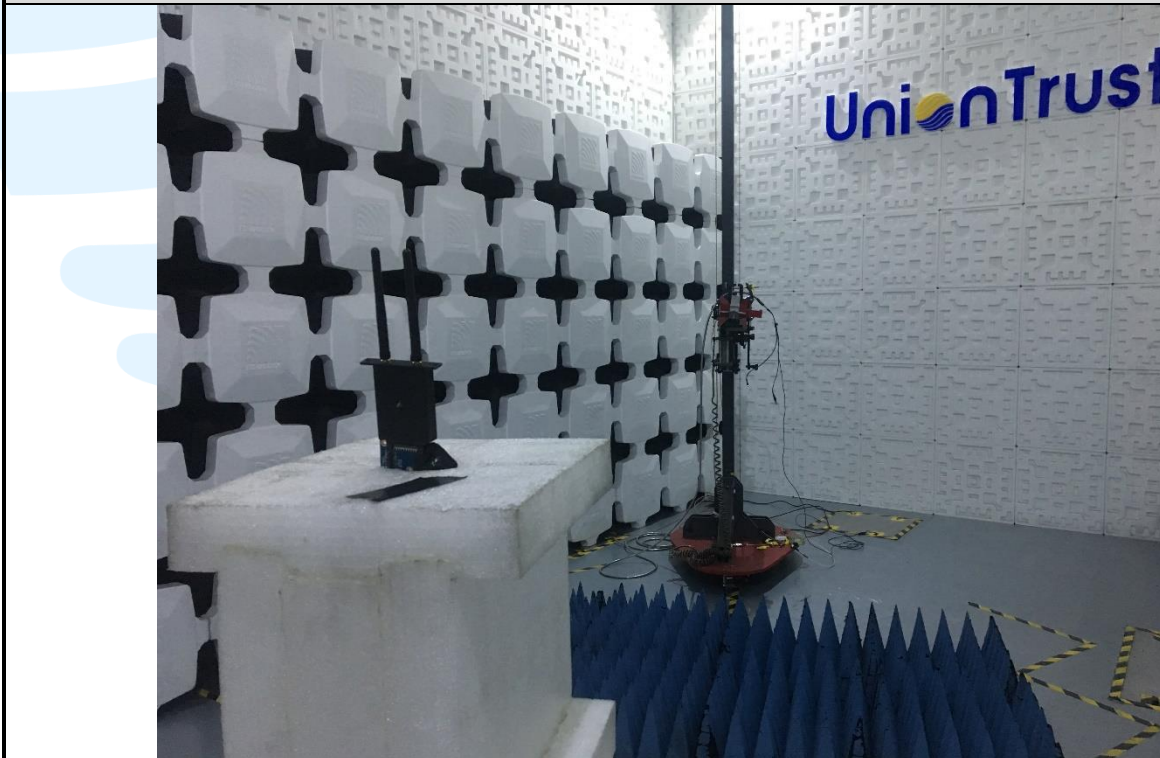
Radiated emission Test Setup (Above 1 GHz)
