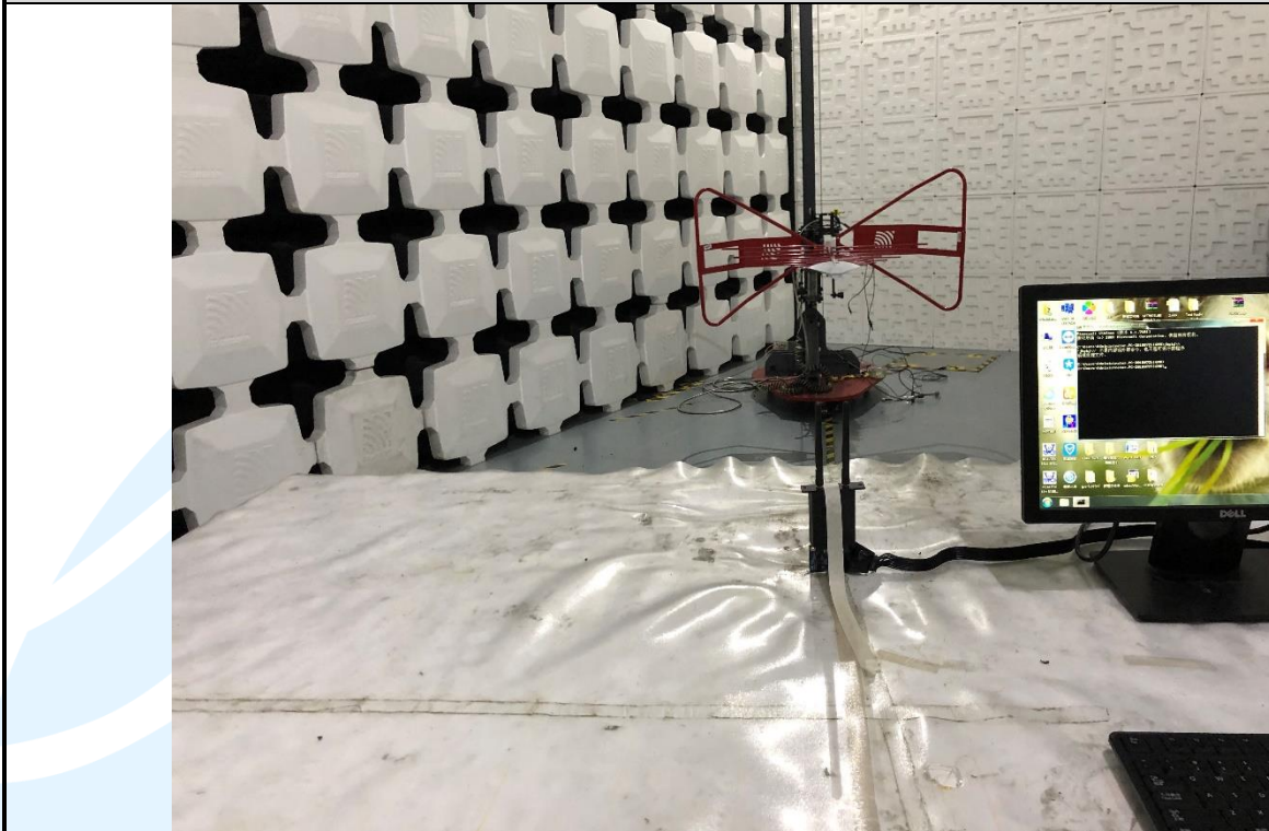
Radiated emission Test Setup (30 MHz~1 GHz)
