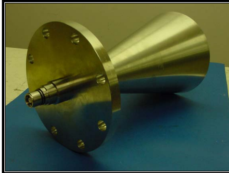
Photograph 26: 21.0 dBi Horn Antenna
