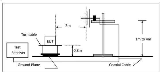
(c) For radiated emissions above 1000MHz
