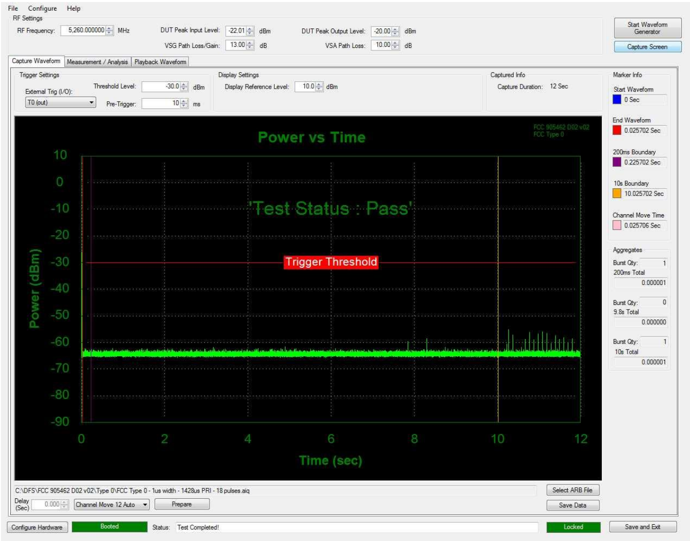
Figure 8.6-1: Channel closing transmission and move time
