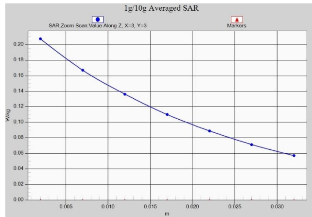
Fig. 1-13 Z-Scan at power reference point (LTE B5 MHz)
