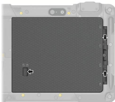
2. Lift the battery pack off the compartment.
