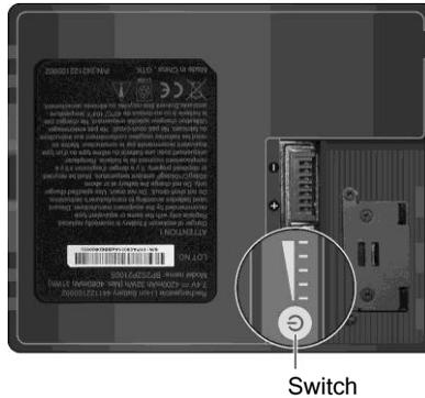
The value of the corresponding green segment indicates the relative percentage of the battery charge. The battery pack is fully discharged when you see no segment glowing green.
