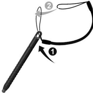
2. Insert the other loop end to the tether holder on the Tablet PC (as indicated by **1** below). Then, insert the stylus end through the loop (as indicated by **2** below) and pull it tight.
