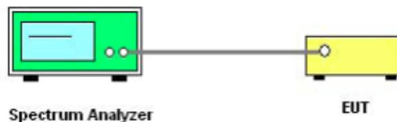
The EUT is connected to the Spectrum Analyzer; the RF load attached to the EUT antenna terminal is 50Ohm; the path loss as the factor is calibrated to correct the reading. Make the measurement with the spectrum analyzer's resolution bandwidth(RBW) = 100 kHz. In order to make an accurate measurement, set the span greater than RBW.
