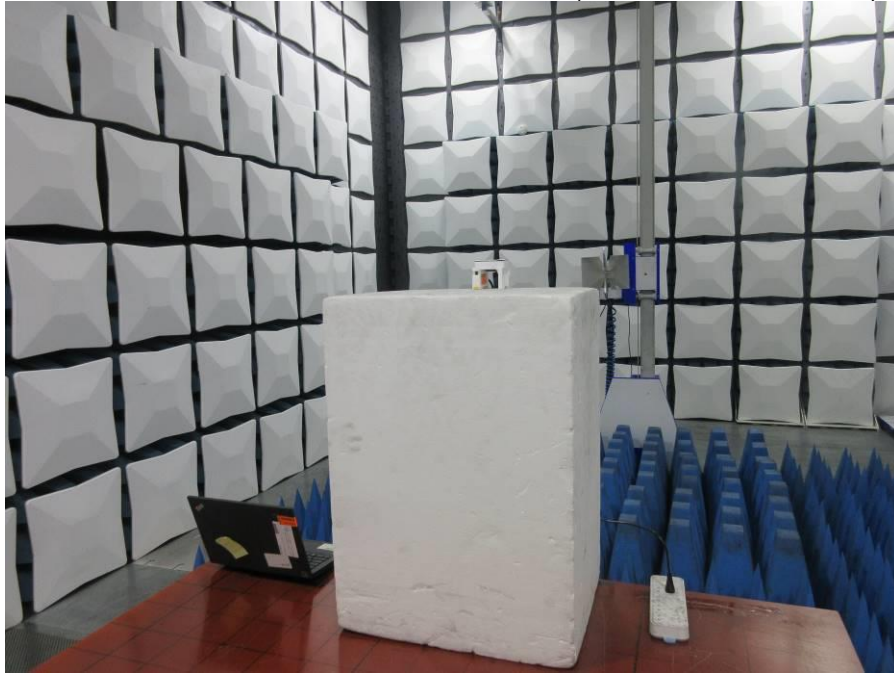
RADIATED RF MEASUREMENT SETUP (ABOVE 1 GHz- Z axis)
