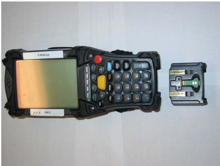
Figure 4 – MC9063 with Battery Removed
