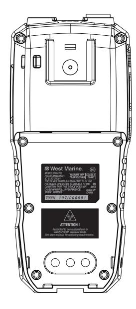
Rating Label for Unit PN:300208968-00001-10 Size:30.3x20.3mm(+/-0.2MM) Material:25# ALUMINIUM LABEL(哑银箔Recycle) Finish:Finish:W/PP Coating Color:sliver text on Black background
