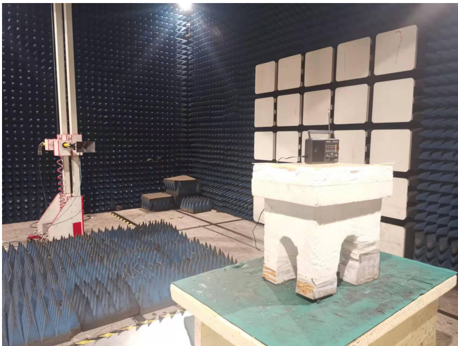
Spurious Emission Test Setup (Above 1GHz)
