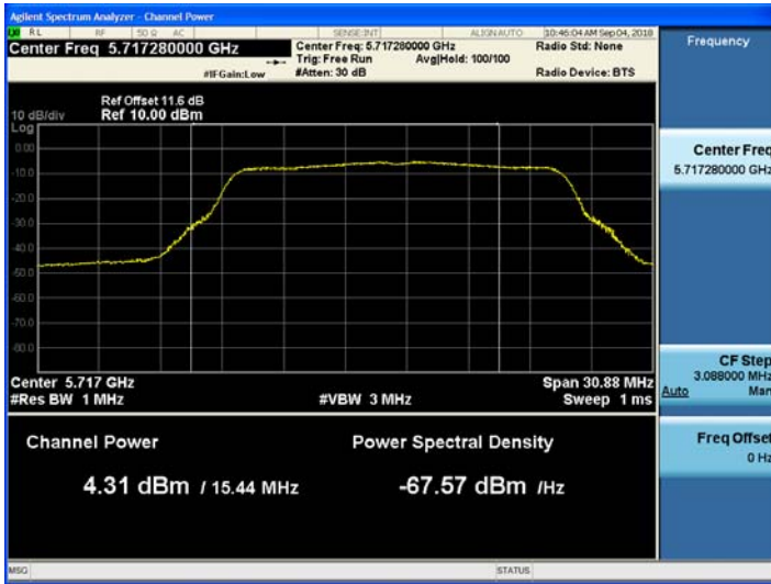
802.11n_HT20 UNII 2C Band Average Power CH.144
