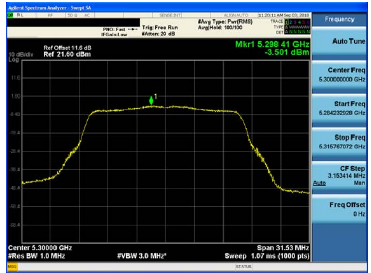
802.11a UNII 3 BAND PSD CH 157
