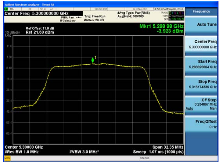
802.11n_HT20 UNII 3 BAND PSD CH 149
