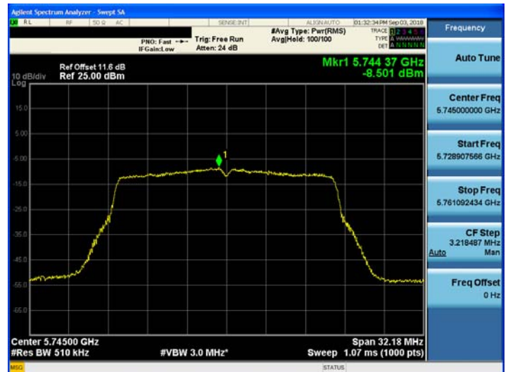
802.11n_HT20 UNII 3 BAND PSD CH 149
