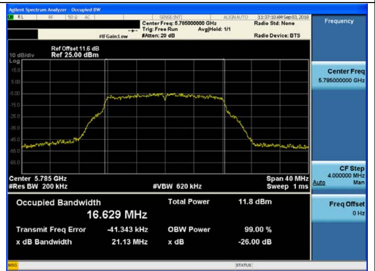
802.11a UNII 3 BAND 26dB Bandwidth (CH 157)
