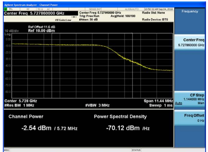
802.11n_HT20 UNII 3 Band Average Power CH.144
