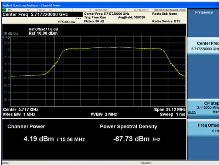
802.11n_HT20 UNII 2C Band Average Power CH.144
