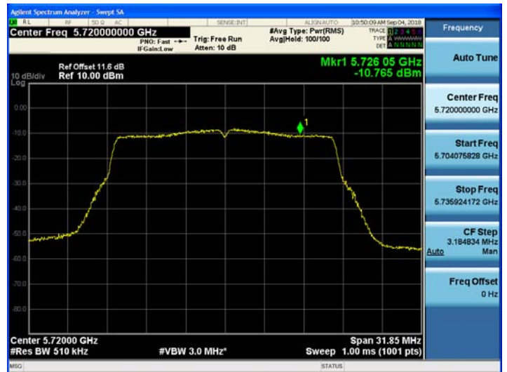
802.11n_HT20 UNII 3 Band PSD CH.144
