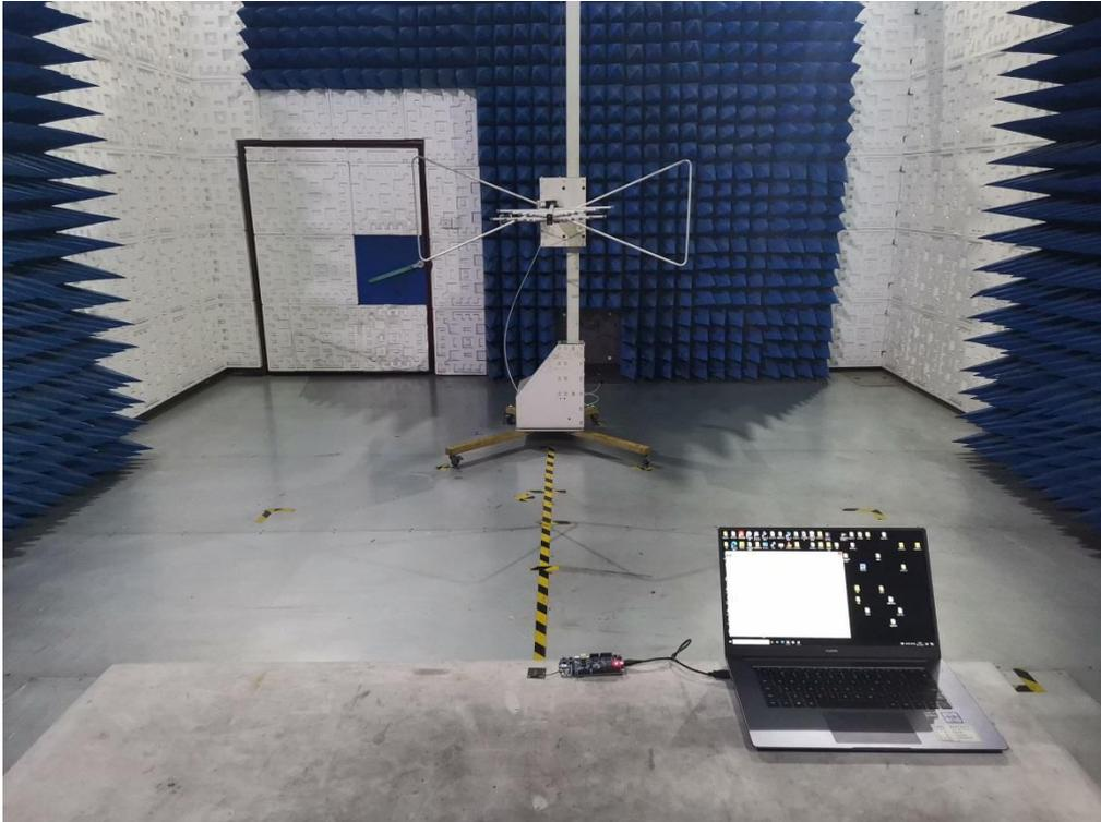
RADIATED EMISSION TEST SETUP BELOW 1GHZ-NORA-B106
