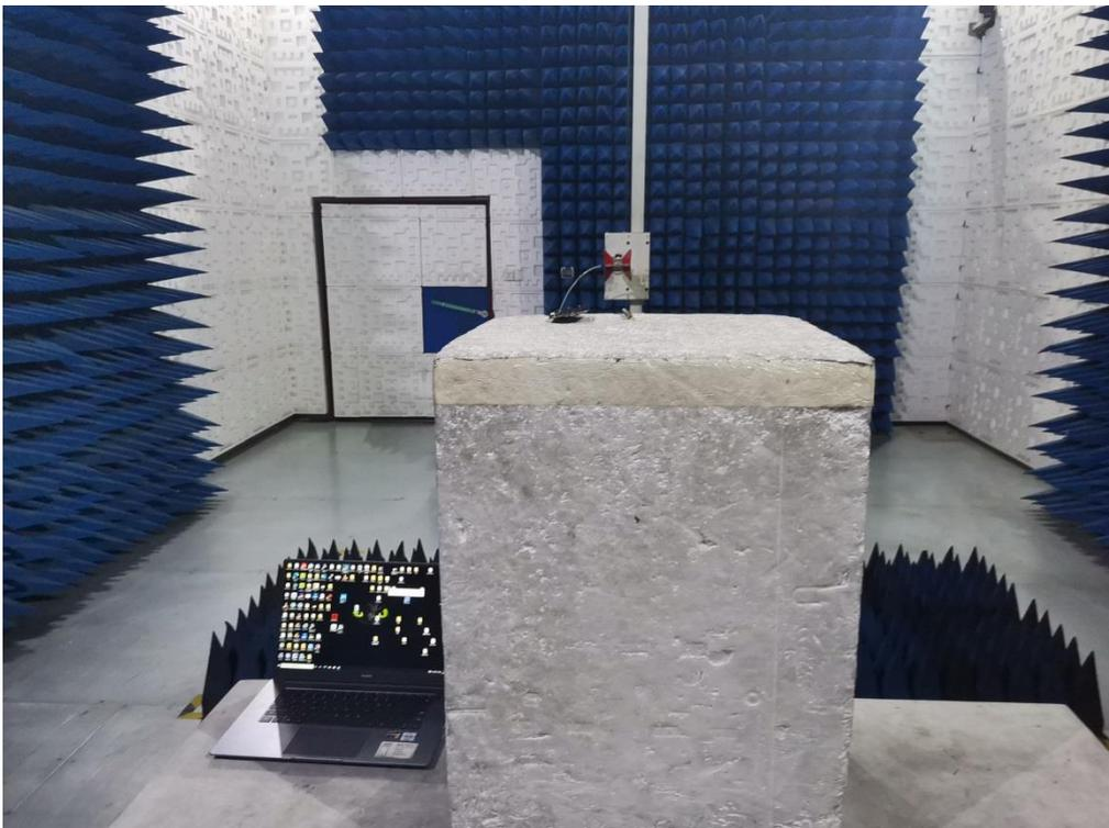
RADIATED EMISSION TEST SETUP ABOVE 1GHZ-NORA-B100 OF ANT 2
