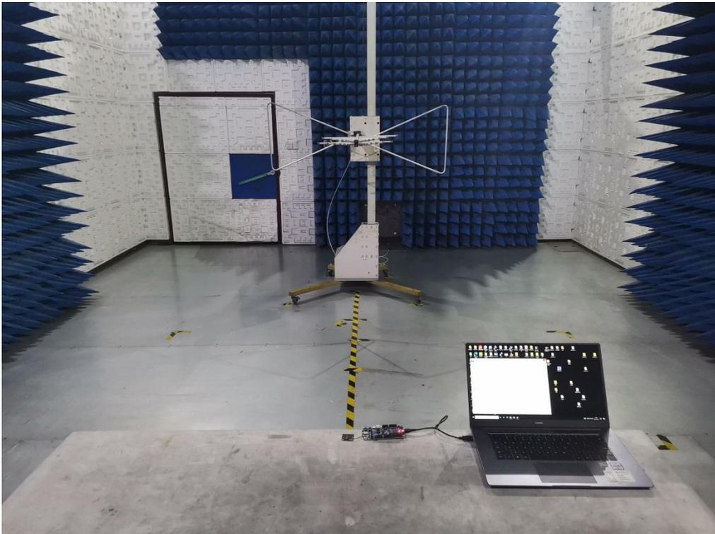
RADIATED EMISSION TEST SETUP BELOW 1GHZ-NORA-B101 OF ANT 1
