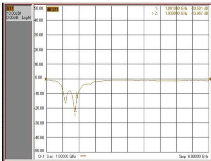
Figure 1: Antenna Return Loss
