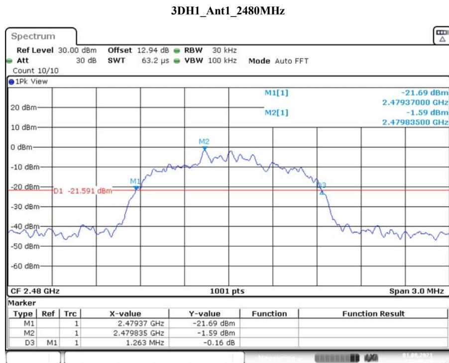
**99% OCCUPIED BANDWIDTH****DH1\_Ant1\_2402MHz**
