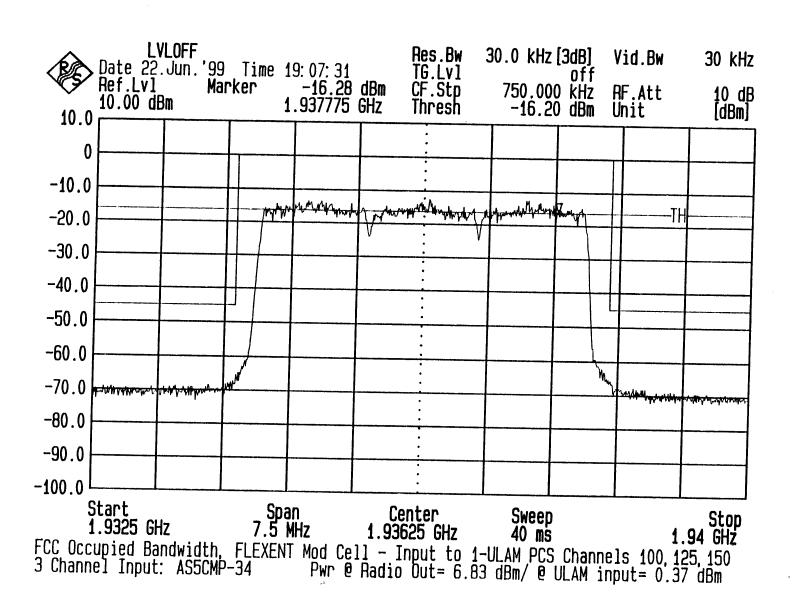
Three Carrier Occupied Bandwidth Block A2
