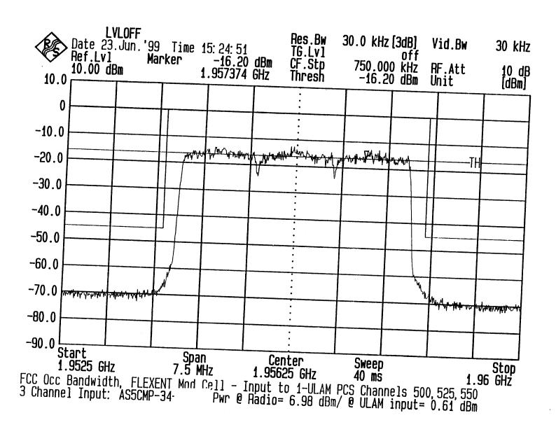
Three Carrier Occupied Bandwidth Block B2
