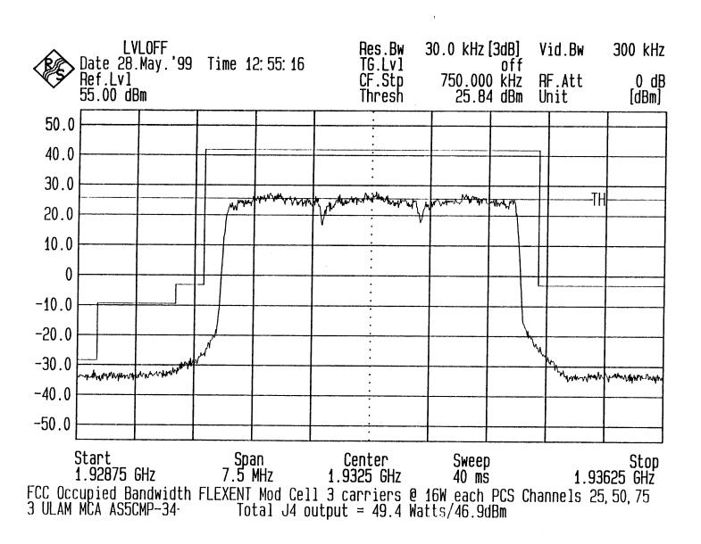
Three Carrier Occupied Bandwidth Block A2
