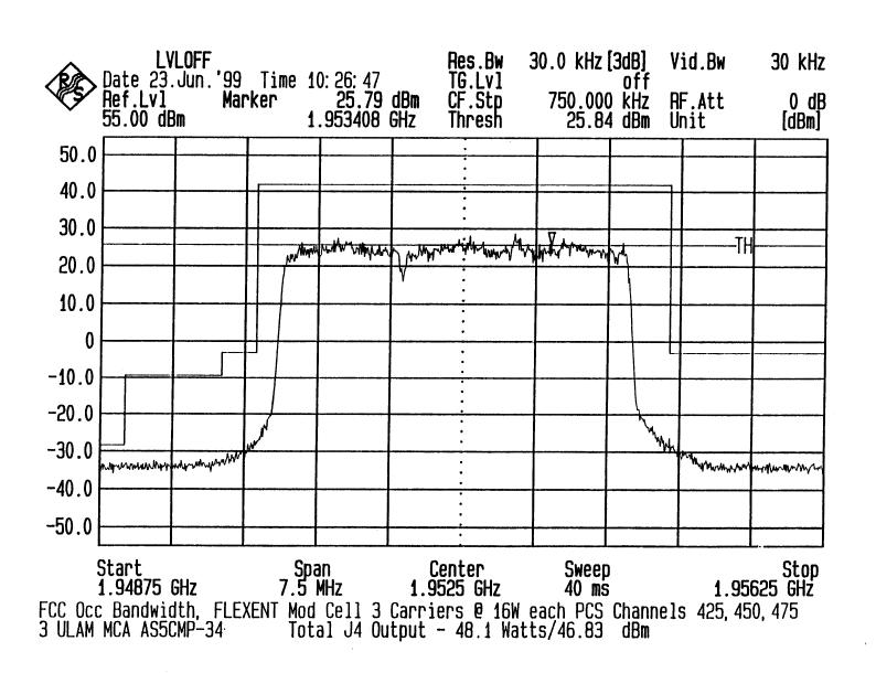
Three Carrier Occupied Bandwidth Block B2
