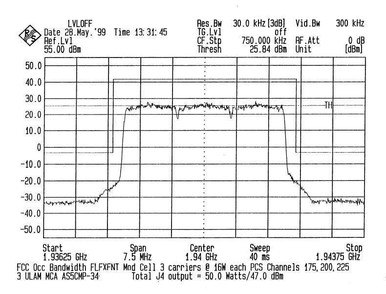
Three Carrier Occupied Bandwidth Block B1
