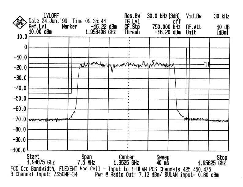
Three Carrier Occupied Bandwidth Block B1
