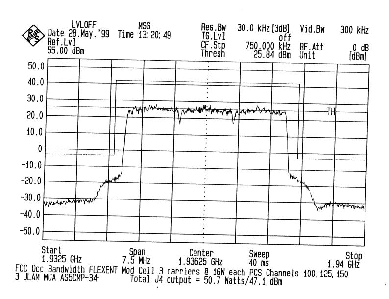
Three Carrier Occupied Bandwidth Block A3
