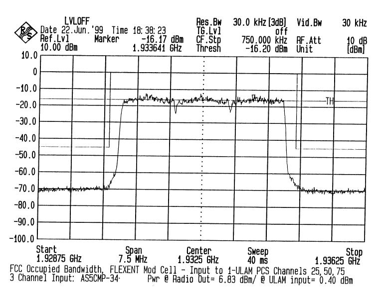
Three Carrier Occupied Bandwidth Block A1
