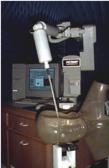
Figure 5. Photograph of the Probe and the Phantom
