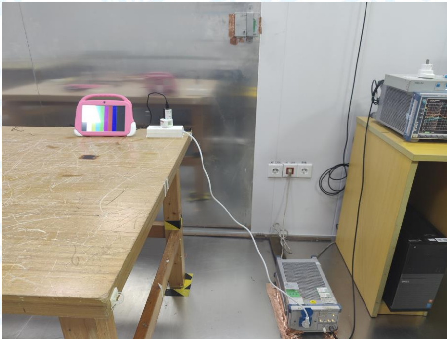
Photo of Setup for Conducted Emission
