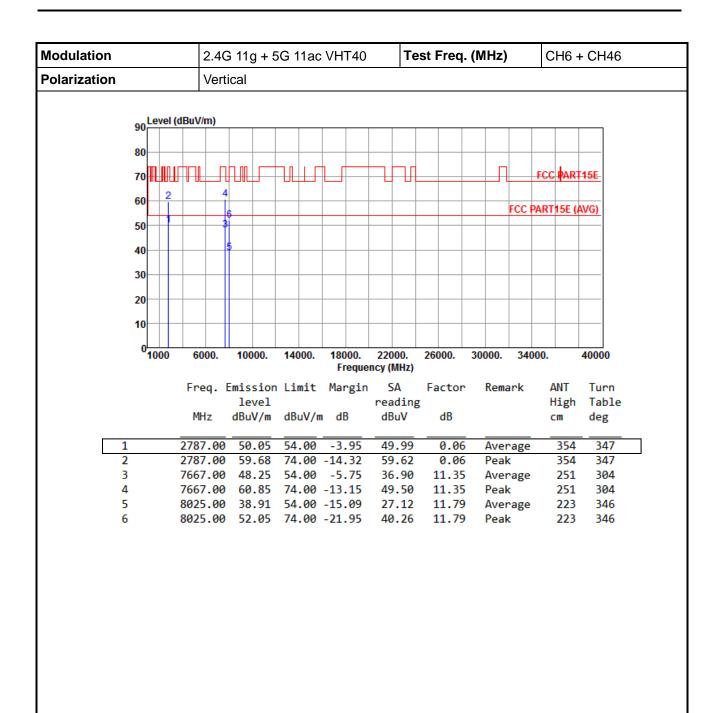
Note 1: Emission Level (dBuV/m) = SA Reading (dBuV/m) + Factor\* (dB)
