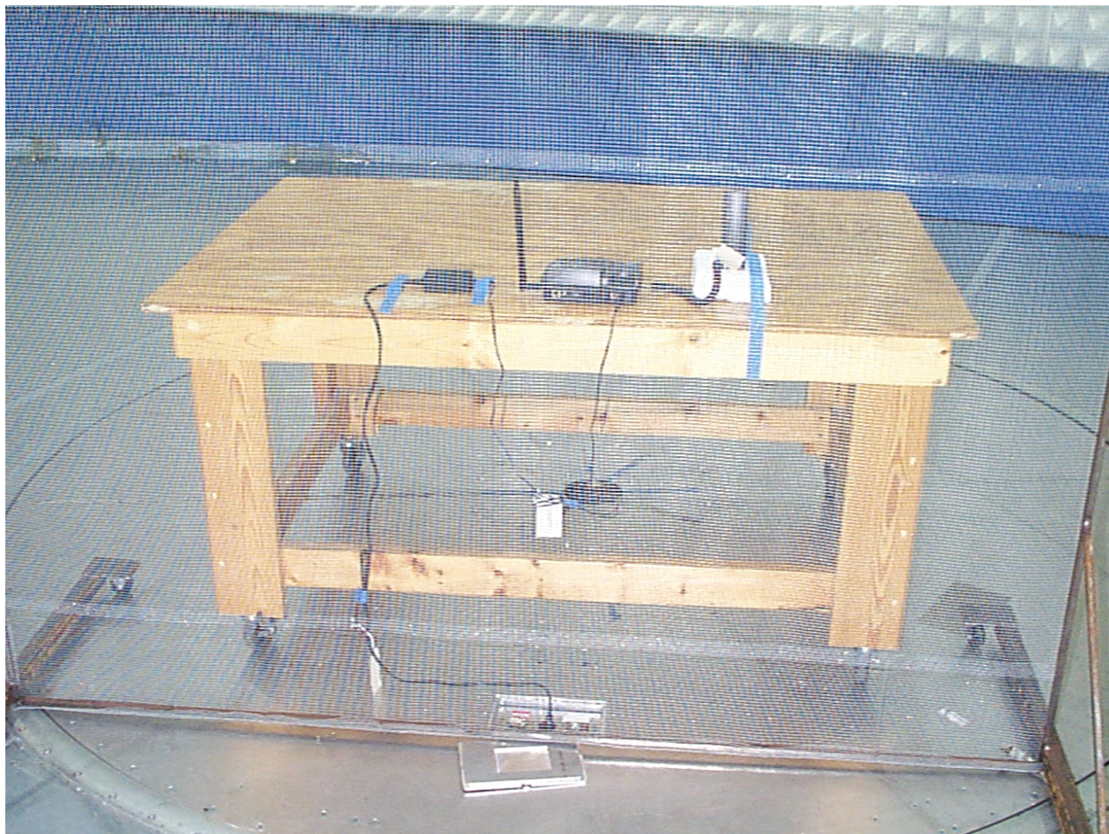
Figure 8-6: Configuration photograph, AC mains conducted emission, rear view
