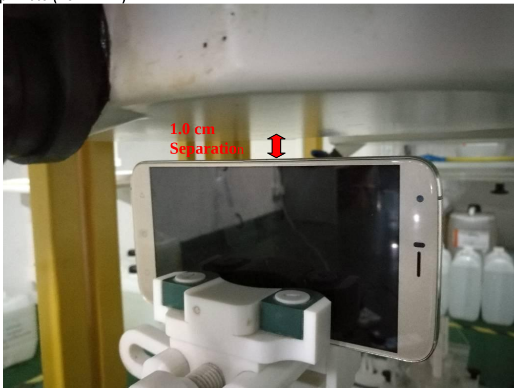
Body Setup Photo (LCD LEFT)
