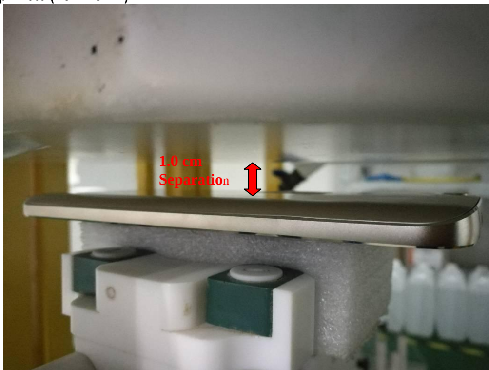
Body Setup Photo (LCD DOWN)
