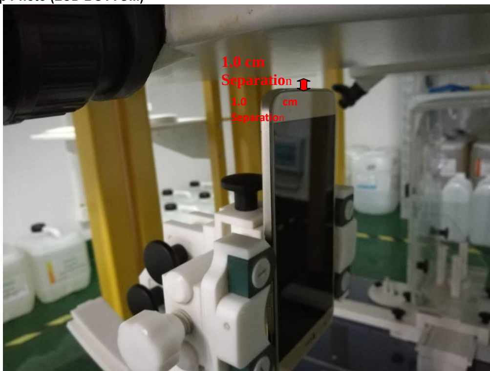
Body Setup Photo (LCD TOP)
