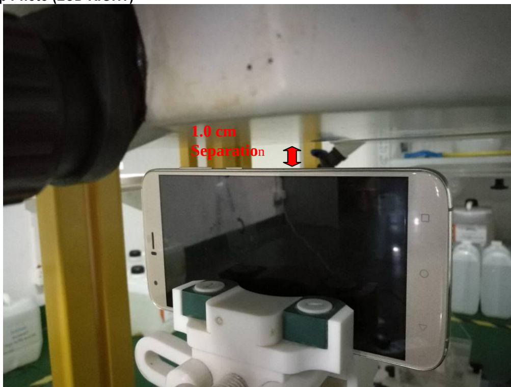
Body Setup Photo (LCD RIGHT)
