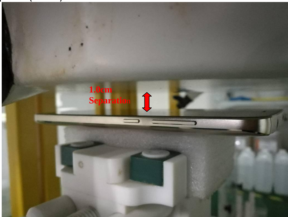
Body Setup Photo (LCD UP)
