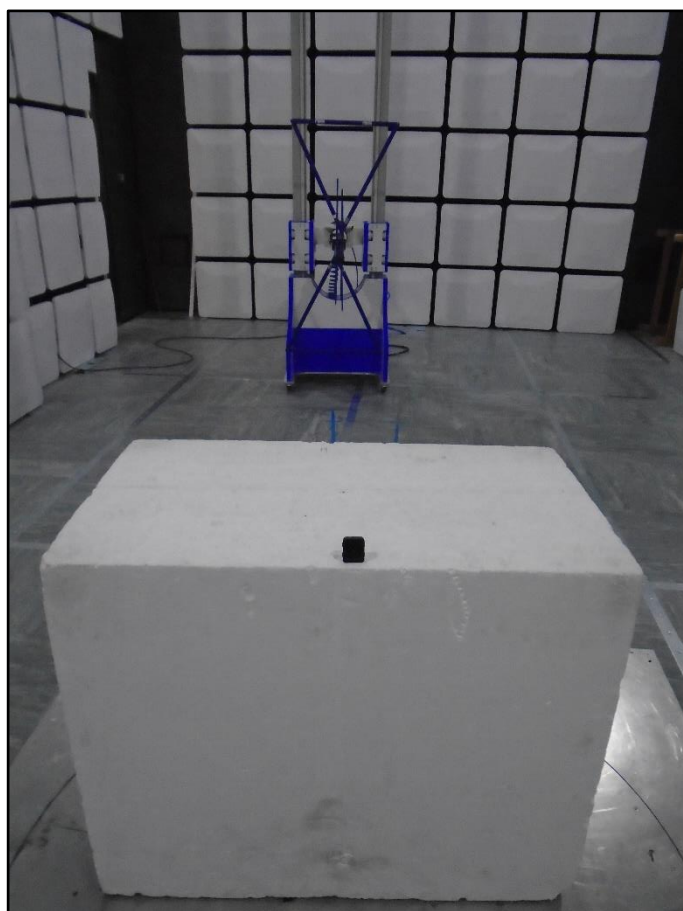
Figure 19 – Test Setup – 30 MHz to 1 GHz, Orientation Y
