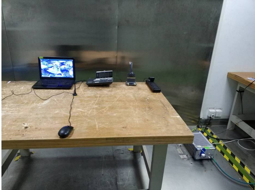
Conducted Emissions - Front View
