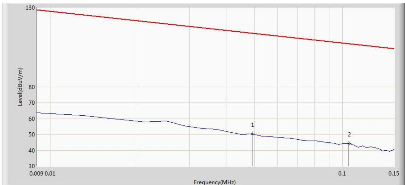
Note: Measure Level (dB $\mu$ V/m) = Reading Level (dB $\mu$ V) + Factor (dB)
