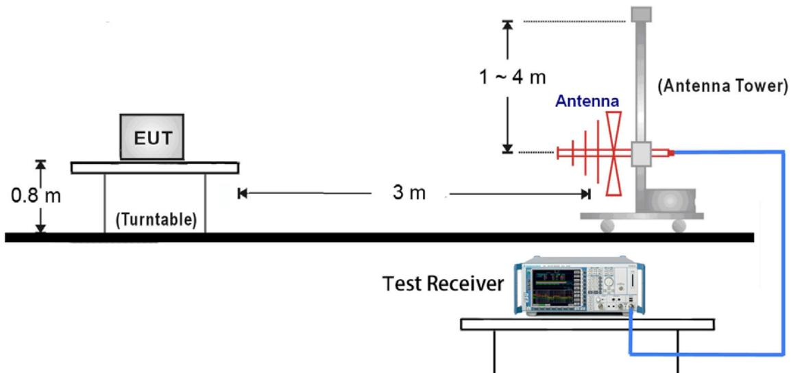
1GHz ~ 25GHz Test Setup:
