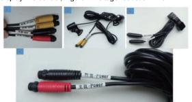
2 , As shown in the following figure: Figure1-Connect the front and rear recording and Type-C adapter with BMW plug and twist tightly; (Note that there is a label on the wire indicating front/rear camera)
