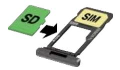
**NOTE:** If you need to reinstall your SIM card, remove the original SIM card from the tray and place your new SIM card into the tray with the gold contacts facing down as shown.
