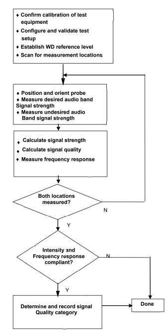
Figure 4-14 C63.19 T-Coil Signal Test Process
