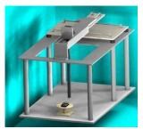
**Figure 4-3** RF Near-Field Scanner
