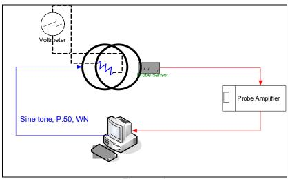
Figure 4-1 Validation Setup with Helmholtz Coil
