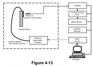
Audio Magnetic Field Test Setup
