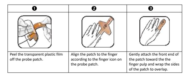
Step 5: Set up the Aulisa Oximeter Module.
